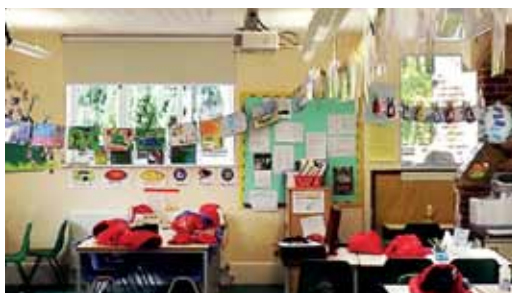
Poor: Small window area, high window height (1.4m), no distant view
